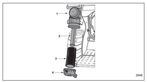
Figure 4-19 Check Engine Air Filter
